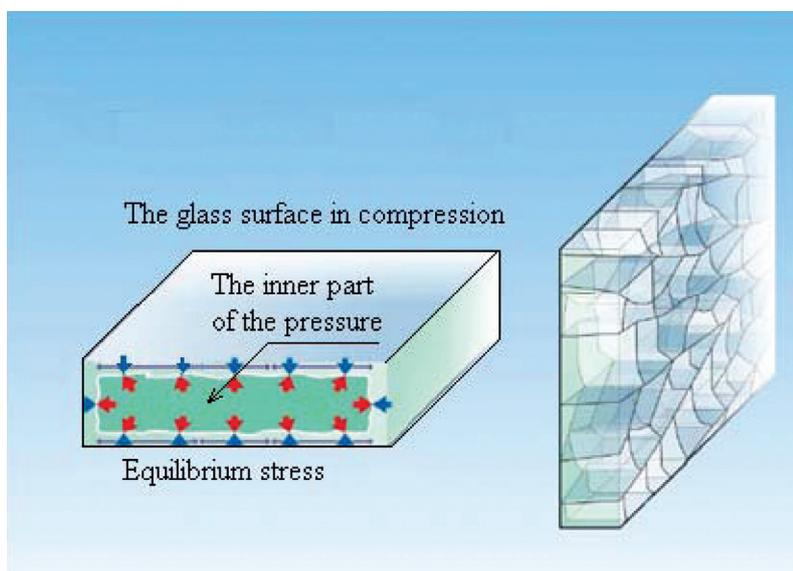
Figure 1 The glass surface in compression
