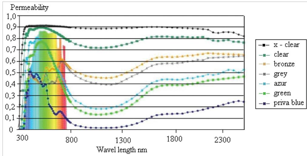
Figure 2 Chart light transmittance of each colored glass version
