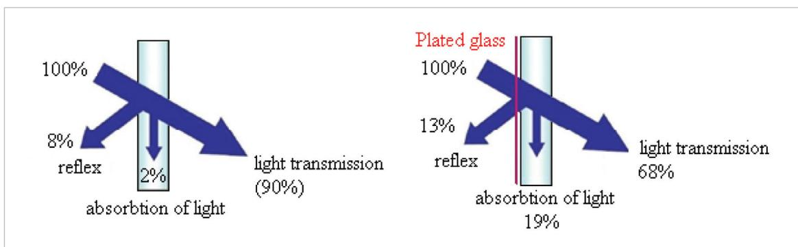
Figure 3 Comparison of light absorption on plated and non plated glass
