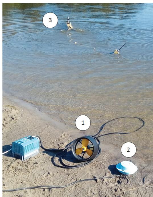
Figure 3 Test stand on the shore of the lake: 1 – propeller, 2 – underwater sound speaker, 3 – BUUV2
