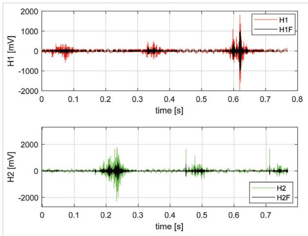
Figure 8 The example of the signals from the both hydrophones before (H1, H2) and after filtering process (H1F, H2F)
