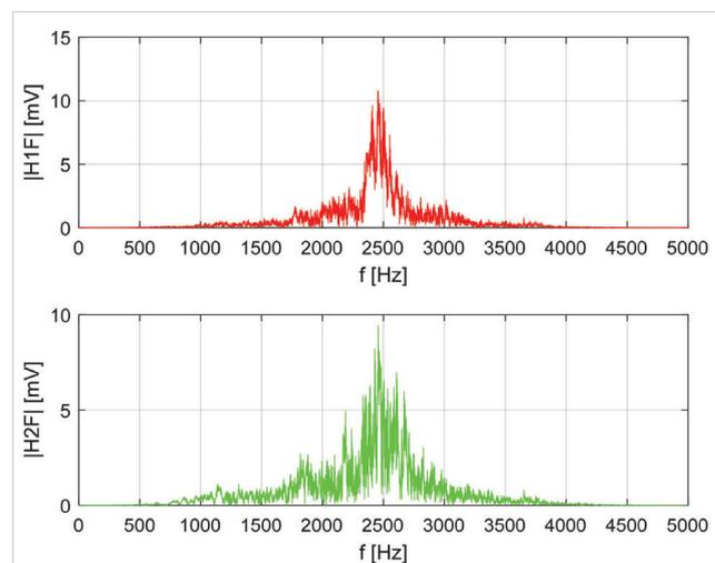
Figure 7 The spectrum of the signal from the front hydrophone (H1) and the rear hydrophone (H2) after filtering process (H1F and H2F respectively)
