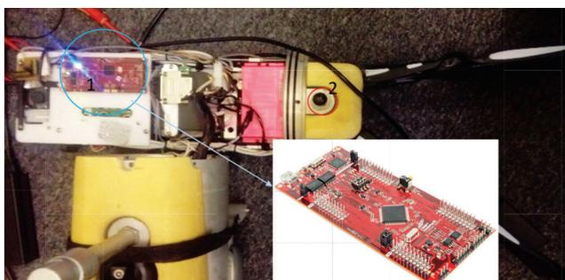
Figure 2 The interior part of the BUUV2: 1- the microcontroller unit, 2 – the rear hydrophone
