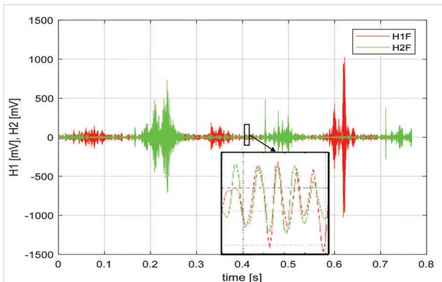
Figure 9 The signals from the both hydrophones represented in the time domain after filtering process
