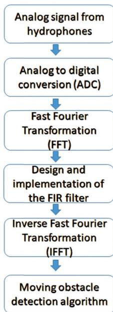
Figure 4 Signal processing algorithm for passive detection of the moving obstacle
