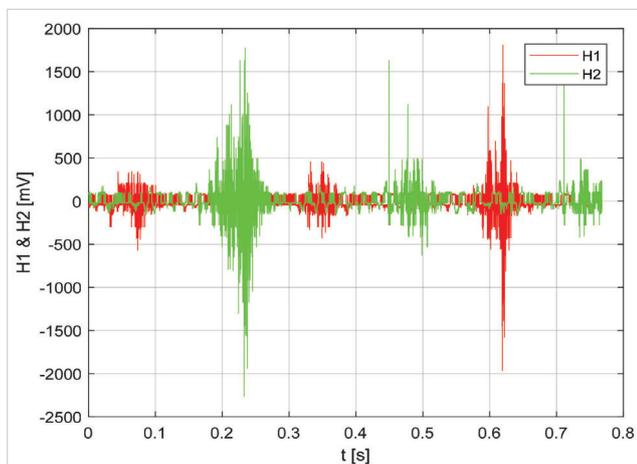
Figure 5 Two signals measured by the hydrophones as a function of time
