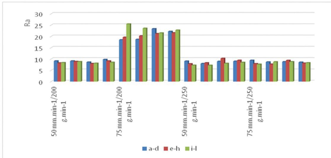
Figure 7 Dependence surface roughness parameters for constant cutting speed and feed abrasives
