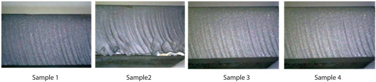
Figure 6 Cutting quality individual samples
