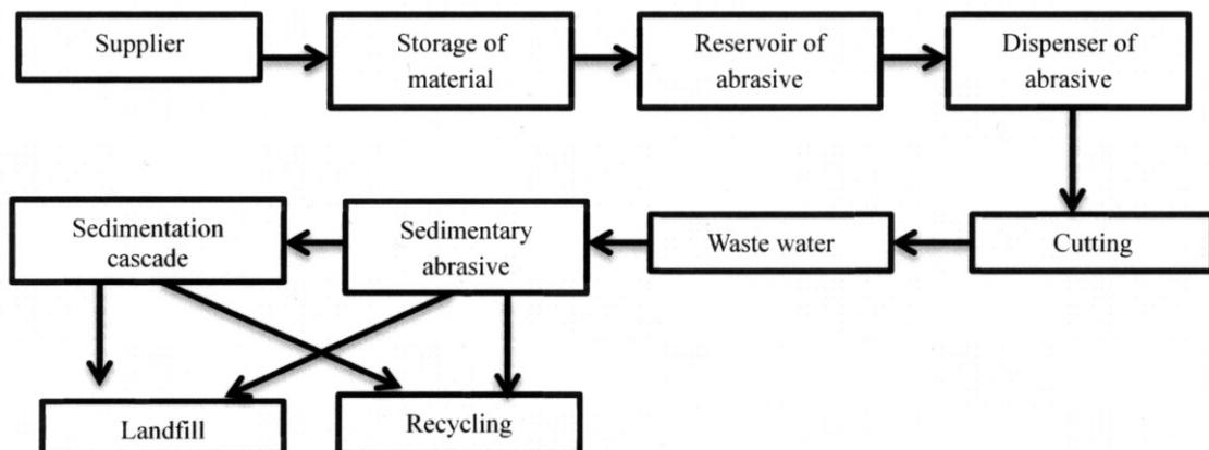
Figure 3 Flow abrasive in the process
