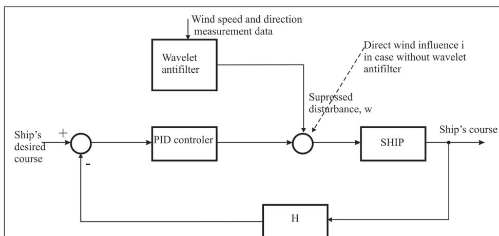
Figure 4. Proposed controller design for wind influence suppression
