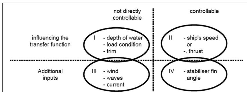
Figure 2. Designations of controllable and not directly controllable inputs and disturbances
