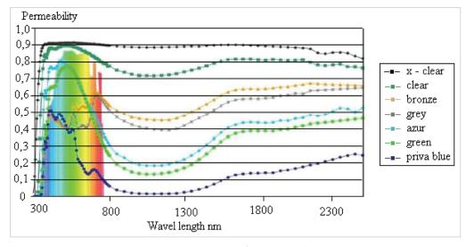
Figure 2 Chart light transmittance of each colored glass version
