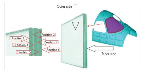
Figure 4 The numbering of the individual positions of the glass sheets
