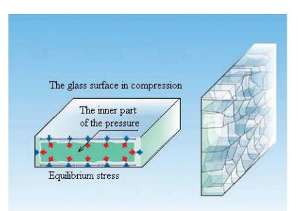
Figure 1 The glass surface in compression
