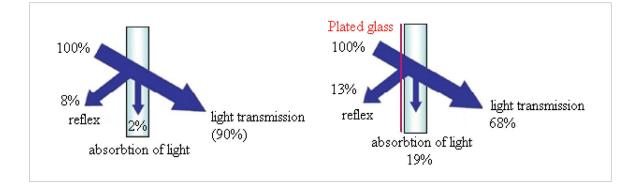
Figure 3 Comparison of light absorption on plated and non plated glass
