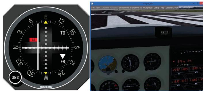
Figure 4 Visualization of the 3D model movements of the indicator on the left, and the actual event during flight as by the FlightGear on the right
