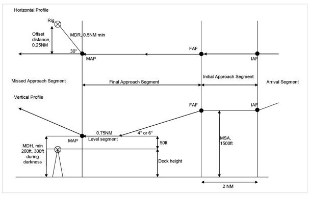
Figure 1 SOAP Approach Plan and Vertical Views Slika 1. SOAP plan pristupa i vertikalni oqledi
