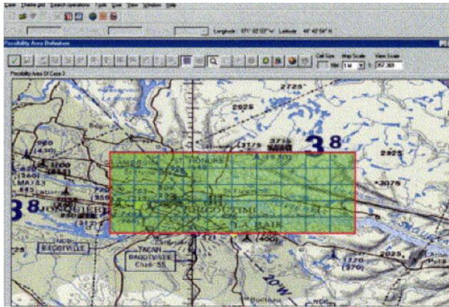
Figure 2 Automatic grid of the possibility area in SARPlan
