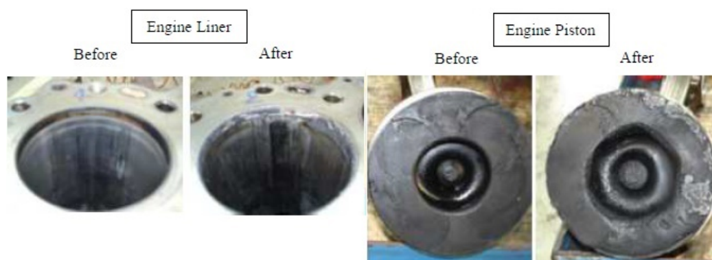
Figure 6 Damaged engine liner and piston due to dual fuel knocking
