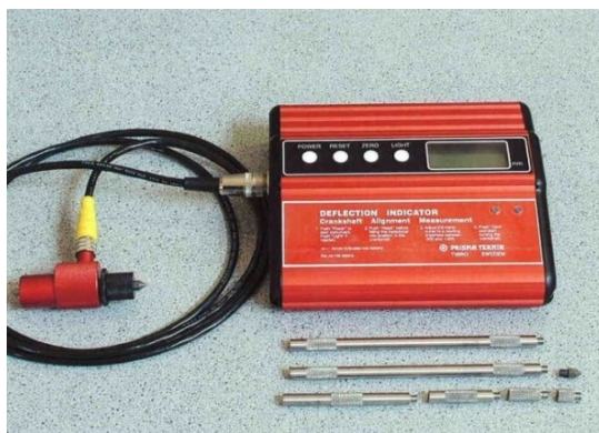
Figure 11 – Deflection gauge with extensions and unit for connection to computer (Source: Deflection Indicator Manual PC)
