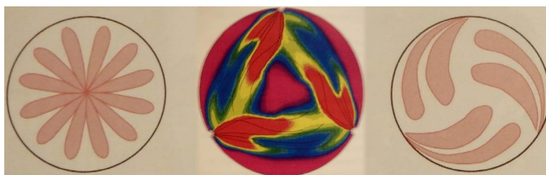
Figure 13 Correct injection spray shapes in the injection flow of a four-stroke trunk-piston engine (left), in a large two-stroke crosshead engine with three injectors (centre), and a two-stroke crosshead engine (right).
