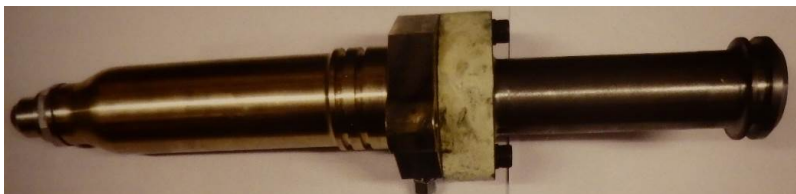
Figure 10 A complete pre-chamber that will be installed in the centre of cylinder head.
