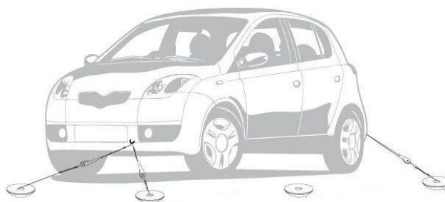
Figure 4 Proper vehicle lashing; Source [8]
