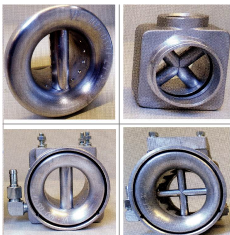
Figure 1 The examples of throat constructions from gas mixers for different engines.
