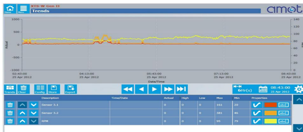
Figure 2 – Curves showing operation of two selected sensors according to rpm (Source: AMOT Software Manual)
