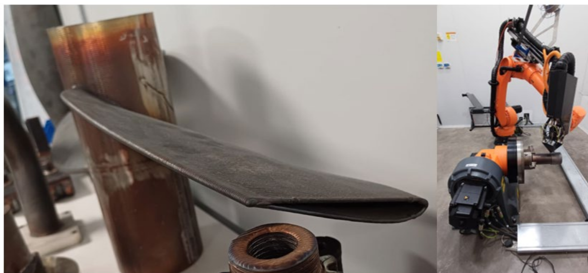
Figure 2 Example of making a ship propeller by a robot equipped with the Meltio Multi-laser IR Deposition Head
