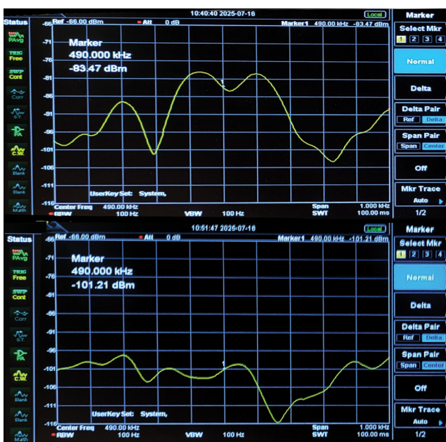
Figure 6 Spectral analysis of signals from Mondolfo (top) and Split (bottom) stations Slika 6. Spektralna analiza signala s postaja Mondolfo (gore) i Split (dolje)
