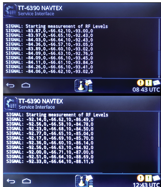
Figure 3 RF Reception Levels from Mondolfo station Slika 3. RF razine prijema s postaje Mondolfo
